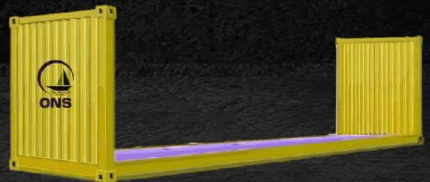
Open top containers are especially suitable for transporting overheight cargo, i.e. cargo taller than 2.54m (8'5"). They are available in two sizes: 20' and 40'. Cargo can be loaded by crane from the top-side. Over height cargo can also be loaded from the door-side since the door header can be swung open.
